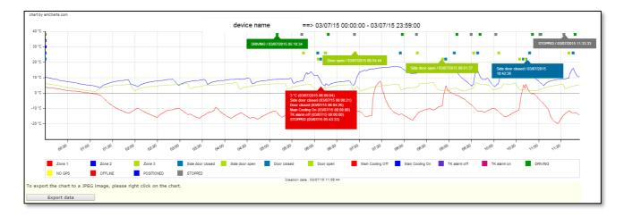
The number of temperature curves depends on the number of installed sensors in the trailer, generally 1 per zone. In this example, we have 3.
